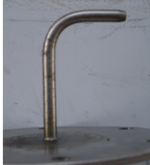
Outlet particulate sample probe after the Venturi scrubber and condenser absorber.
