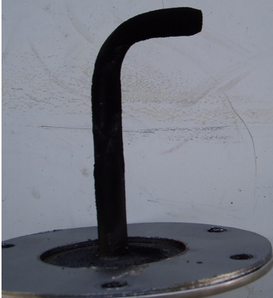
Inlet particulate sample probe before the Venturi scrubber.
