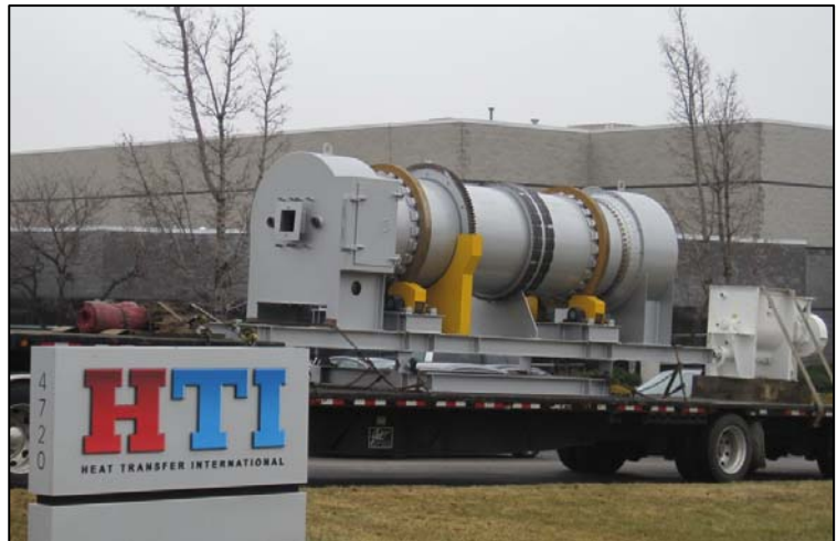
HTI Rotary Kiln Gasifier
