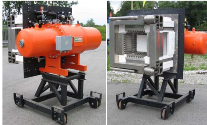
Figure 6. Front and back view of the 35 kW el Stirling engine developed for biomass CHP plants including the heater forming an interface to the combustion chamber
