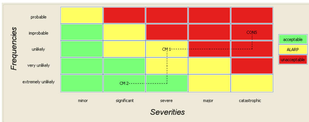
Figure 4-4 Risk matrix for the characterisation and visualisation existing and/or remaining risk potentials
